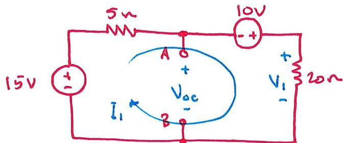
$$I_1 = \frac{15V + 10V}{5\Omega + 20\Omega} = \frac{25V}{25\Omega} = 1A$$
