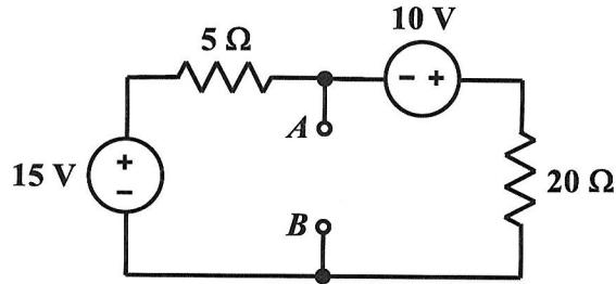
Determine the Norton equivalent circuit with respect to terminals *A* and *B*.
